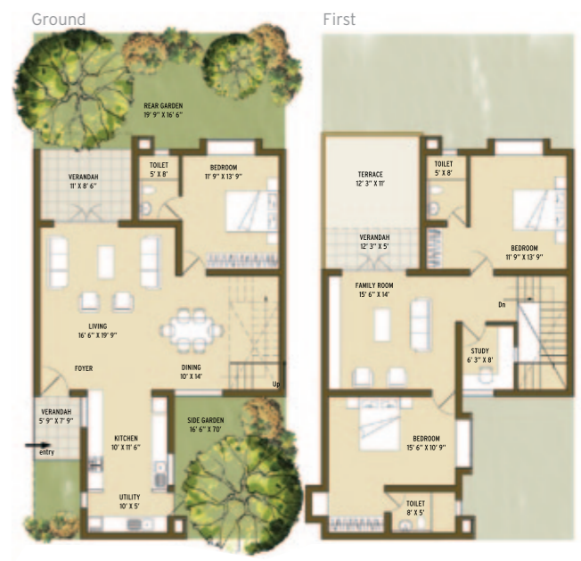
TYPE 4B Plot area: 2110 sq. ft. Ground floor area: 1170 sq. ft. First floor area: 1130 sq. ft. Total floor area: 2300 sq. ft.
