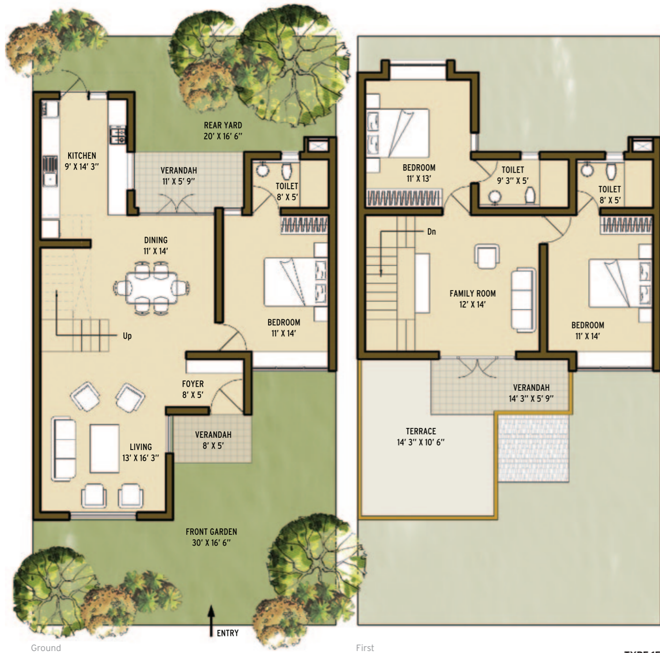
Ground First TYPE 1E Plot area: 1810 sq. ft. Ground floor area: 1050 sq. ft. First floor area: 860 sq. ft. Total floor area: 1910 sq. ft.
