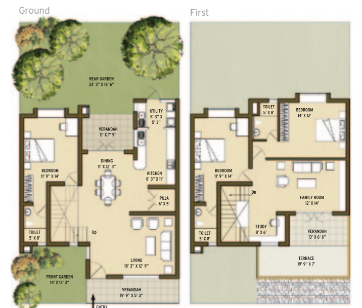
TYPE 1F Plot area: 2000 sq. ft. Ground floor area: 1250 sq. ft. First floor area: 1050 sq. ft. Total floor area: 2300 sq. ft.
