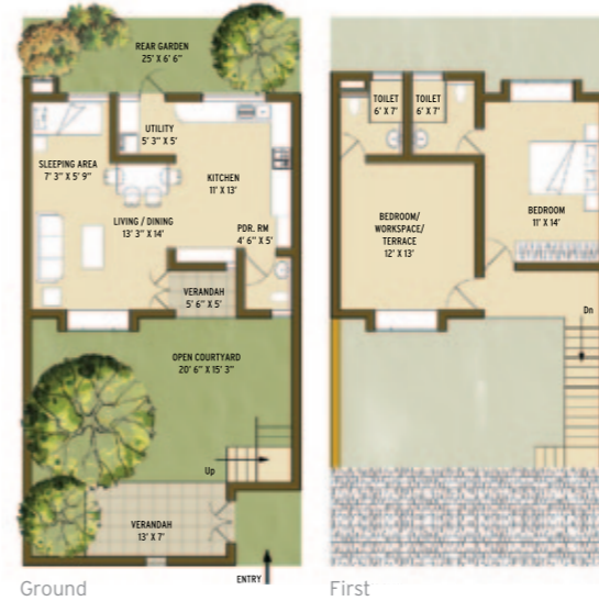
TYPE 2A Plot area: 1250 sq. ft. Ground floor area: 730 sq. ft. First floor area: 575 sq. ft. Total floor area: 1305 sq. ft.
