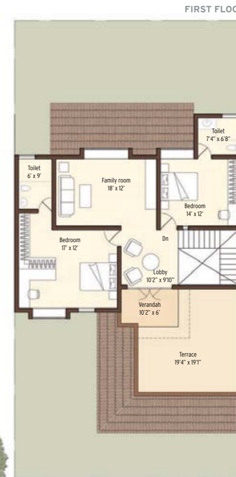
TYPE 1D Plot area: 3215 sq. ft. Ground floor area: 1855 sq. ft. First floor area: 1175 sq. ft. Total floor area: 3030 sq. ft.
